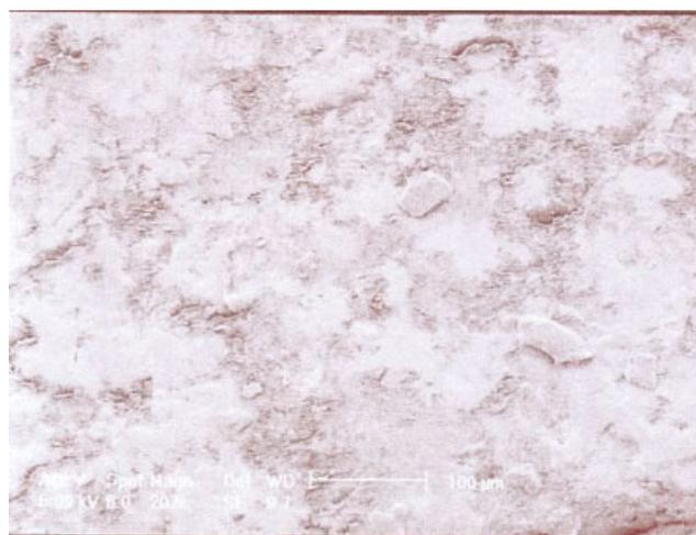
**Figure 12** Scanning electron micrograph showing fractured surface of the adhesive joint when PBI surface is modified by low-pressure plasma and the joint is exposed to high-energy radiation (magnification  $\times 300$ ). [Color figure can be viewed in the online issue, which is available at [www.interscience.wiley.com](http://www.interscience.wiley.com).]
